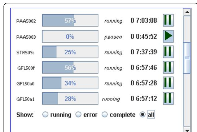
**Figure 2 Monitoring jobs in Auto-SAM.** We implemented a job-monitoring system that regularly checks the progress of each job in the database. Using this monitor, the analyst can follow each job's progress, request error information, and pause and kill jobs. This job monitor is integrated into GenAMap.
